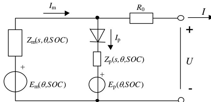
Figure 3. A generic electrical network often used to model electrical behaviour of different kinds of batteries.
