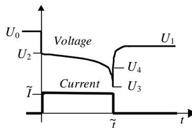
*Figure 14. Evaluation of battery parameters from step response.*
