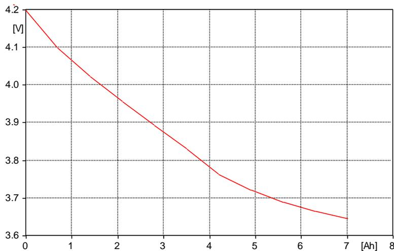
Figure 9. OCV-SOC correlation for a lithium battery, from results of fig.8 .
