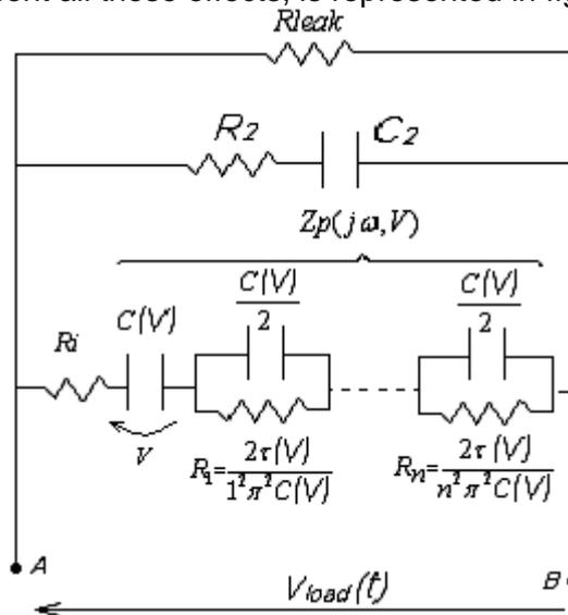
Figure 12. Complete electric model of Supercapacitors.
