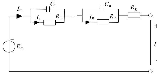
Figure 5. Electric network applicable when parasitic reactions are absent (parameters depend in general on SOC and inner battery temperature).
