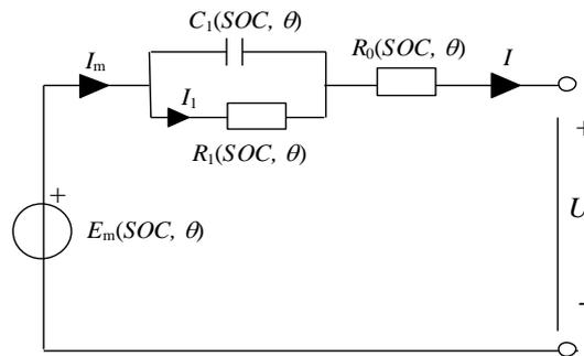
Figure 6. Electric network chosen for HCV lithium battery modelling (dependence on SOC,  $T$  and numerical parameters to be determined based on lab tests).
