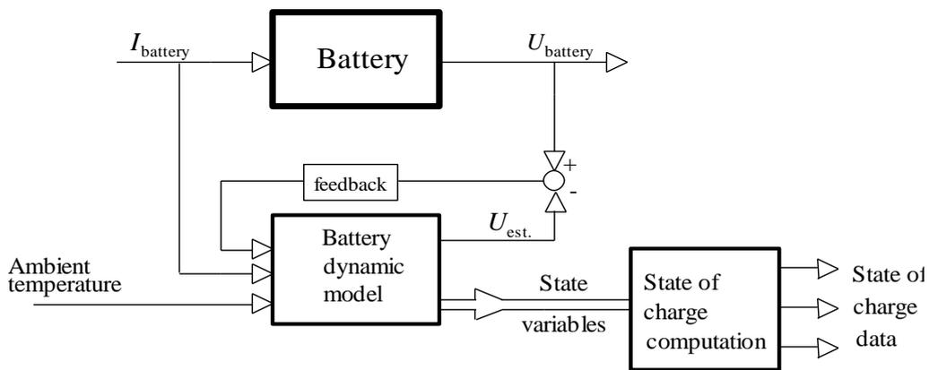
*Figure 7. Principle scheme of a Luenberger battery state observer.*
