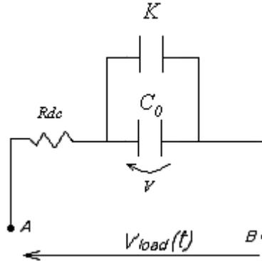
*Figure 13. First branch model for frequencies tending to  $10^{-2}$  Hz.*
