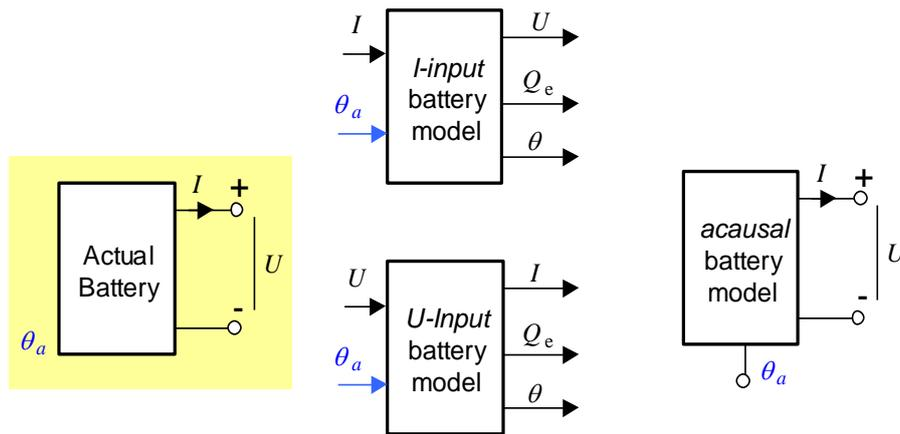
*Figure 1. Different kinds of models of the battery's electric behaviour.
