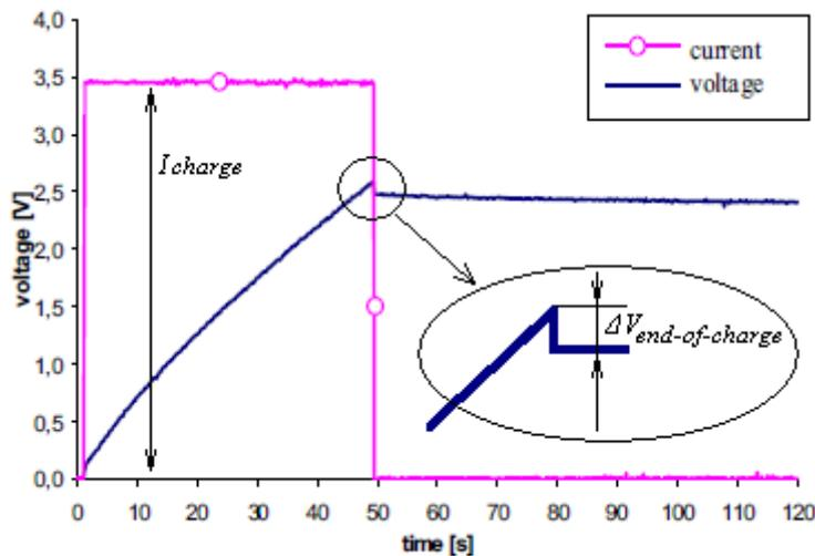
Figure 15. Supercapacitor terminal voltage charging at constant current.
