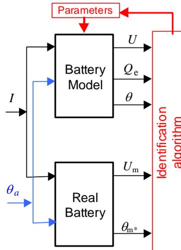
Figure 2. Parameters identification for a model of battery electric behaviour.
