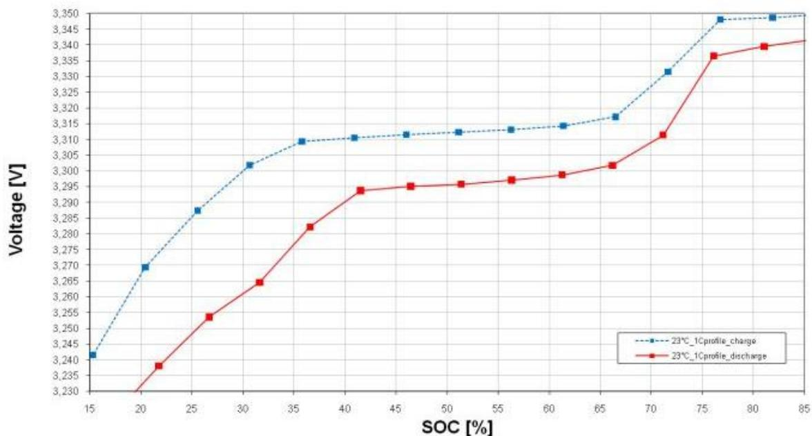
Figure 10. OCV-SOC correlation curves for some Magna Lithium batteries.
