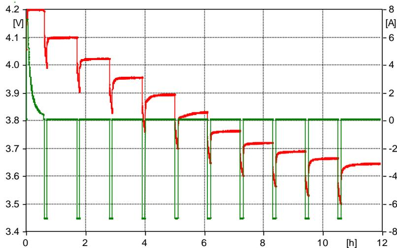
Figure 8. The discharge-based Multiple-Step Test.
