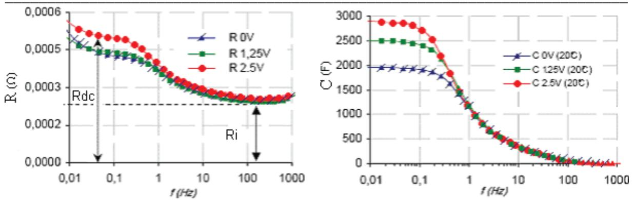
Figure 11. Frequency response of Maxwell BCAP0010 cell (2700F@2.7V).
