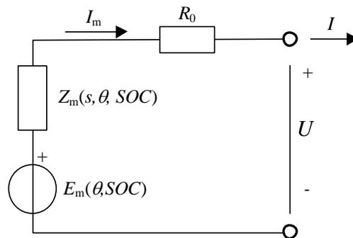
Figure 4. Simplified battery electric equivalent (neglecting the parasitic reactions).
