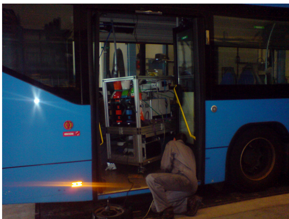
Figure 3: Measurement equipment being installed in the hybrid bus.
